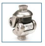
Variable friction offers increased resistance as the knee bends from full extension, providing variable walking speeds. A disadvantage of variable friction is this system requires frequent adjustments and repair to moving parts and is considered less advanced than fluid control knee systems.
