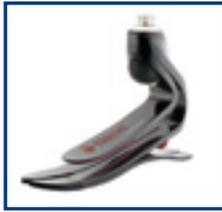
Thrive utilizes a synergistic, dual-keel design incorporating a full-length primary keel and a secondary load-activated keel. When an additional load up to 30 percent of the user's body weight is sensed, Thrive's primary keel progressively comes into contact with the upper keel, providing incremental support. This ensures consistent performance and ultimately greater confidence among users.
